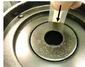
Fig 2: The arrow shows the gap where the voice coil moves up and down in a magnetic field
