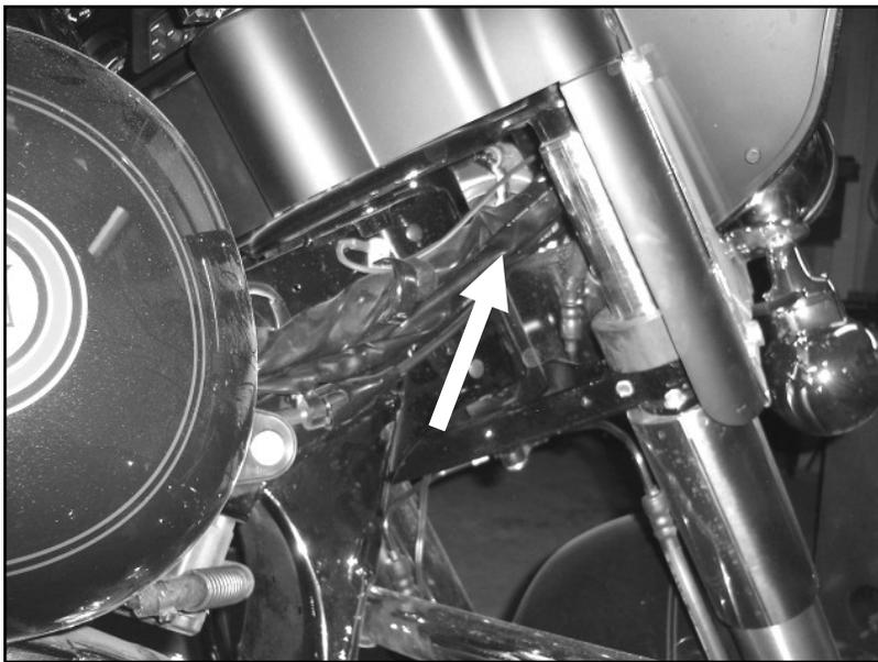
**Diagram 1.4** Stock Harness and Power Harness Passing From Fairing To Under Tank. Note: Harness will pass over front gas tank mount/ bolt. The rings on the power harness can easily scratch paint so **PLEASE** be careful!
