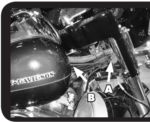
Figure 1.3 - Stock Harness and Amplifier's Harnesses Passing From Fairing To Just In Front Of Tank (Arrow A). Cable Tying the 2 Amp Harnesses To The Main Bike Harness Just In Front Of The Tank (Arrow B) Allows The Amp Harnesses To Go Up Towards The Tank's Chrome Console Easier And Makes For a Cleaner Install.
