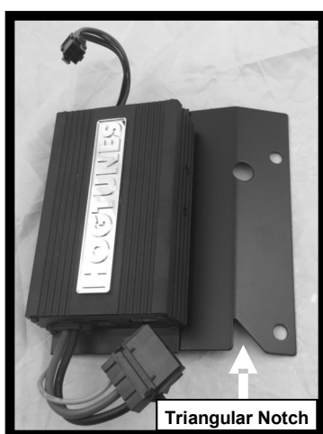
Fig 1.2: REV 200-AA amp Correctly positioned on adaptor plate
