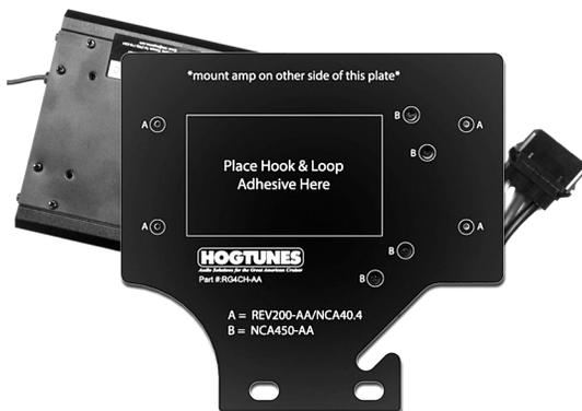
Step 2) Put the plate over the amp as shown above and reinstall 4 screws into holes marked "B". Apply 1 side of hook and loop in area shown on plate.
