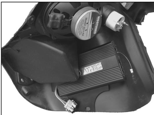
Step 3) Clean area on inner fairing where other half of hook and loop adhesive will go. The bolts that hold the turn signals in place will secure the plate even though the adhesive does most of the work. Plug the supplied power harness extension into amp and follow amplifier manual for wiring instructions.
