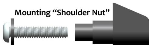
**Step#3: Mounting the Control Box:** The control box can be mounted anywhere on the bars, but careful consideration must be given to the operator safely adjusting the control buttons while the machine is still or in motion. The kit comes with “collars” that adapt the handlebar clamp to fit 7/8”, 1”, or 1.25” diameters and only fit one way. As shown below, the screw that must be used closest to the ball socket is the longer
