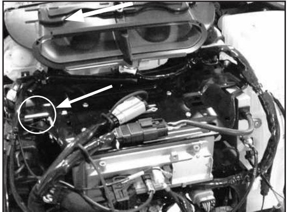
Figure 1.1 - The white circle shows the new location for GPS Antenna if your bike came factory equipped with this feature.
