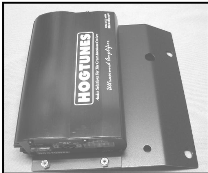
Fig 1.1: Amp positioned on adaptor plate
