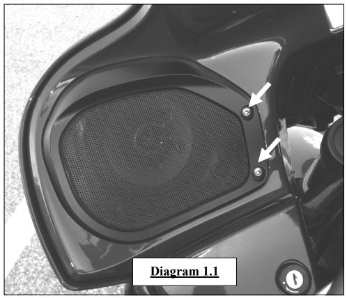
**<u>Step#1:</u>** Remove the 2 screws highlighted by the arrows as shown in Diagram 1.1 above. Carefully remove the grill from the bike.
