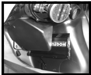
Fig 1.2: NCA 40.4 Amp and adaptor correctly installed
