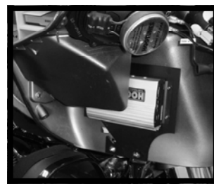
Fig 2.2: NCA 70.2 Amp and adaptor correctly installed
