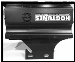
Fig 1.1: NCA 40.4 Amp positioned on adaptor plate
