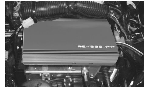
Fig 1.2 Ultra Classic with amp on top of factory CB Module
