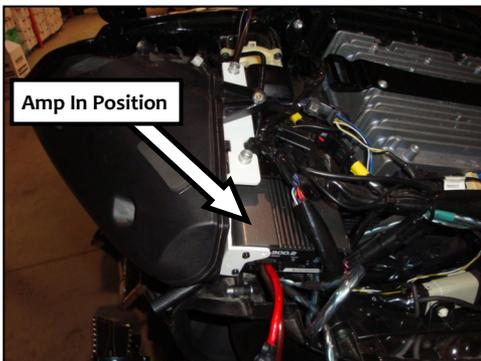
**Step #7:** The holes on the top of the plate mate with the screw holes on the top of the speaker cabinet (bolt holes in Fig 1.2) Holding the amp in position, slide the cabinet/amp into position noting that the amp plate sits over TOP of the factory metal plate. When correctly in place, the factory screws will go
