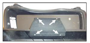
Remove the 4 screws (highlighted with white arrows above) that hold the cloth flap in place. With the flap off, slide one of the metal bars out from inside the flap as it will be used for new lid. The screws just removed will be re-used.
