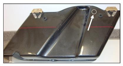
The white circle in the picture above is where a 3/4" (19mm) hole will be drilled. This hole is where the supplied Hogtunes rubber grommet will go, and allow the speaker wire for the lid to pass into the saddlebag.
