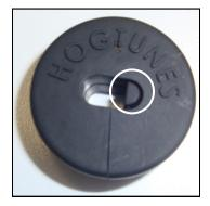
The supplied grommet is "split" to make installation much easier once the wire is in the bag. In the above picture, the white circle is showing a "plug" that can easily be removed. If the only wire you have going into your saddlebag is the speaker wire, leave the plug in place. If you have a second wire for such things as USB power, or a music device interface, removing the plug from the grommet will allow the second wire to also pass without having to drill additional holes in your saddlebag.
