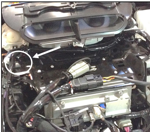
Fig 1.1: The white circle shows the new location for GPS Antenna if your bike came equipped with this feature.
